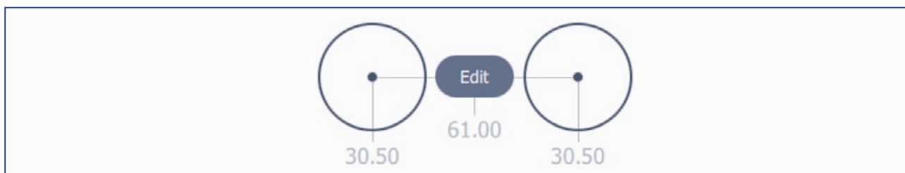
Fig 4. Example of measured distance between optical centres; 30.5 mm left and 30.5 mm right with a total of 61.0 mm
